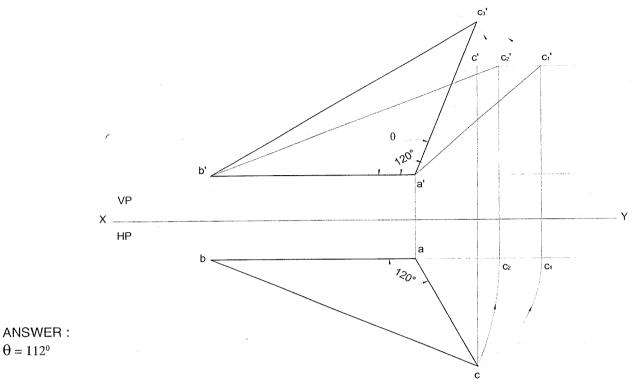
**Problem 40** The elevation of a line AB 90 mm long, is inclined at 30° to HP and measures 70 mm. The end A is 20 mm above HP and is in VP. Draw the projections of the line and find its inclination with VP. **Solution**
