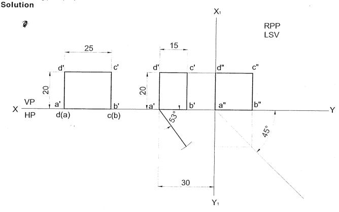
**Problem 16** The front view of a rectangular lamina of sides 30mm x 20mm is square of 20mm sides. Draw the projections and determine the inclinations of the surface of the lamina with HP and VP.
