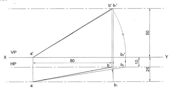
**Problem 47** A straight line PQ 80 mm long appears to a length of 50 mm and inclined at 30% to xy line in its top view Draw its projections when its end point P is 15 mm above HP and 60 mm infront VP. Point Q is nearer to VP than P. **Solution**
