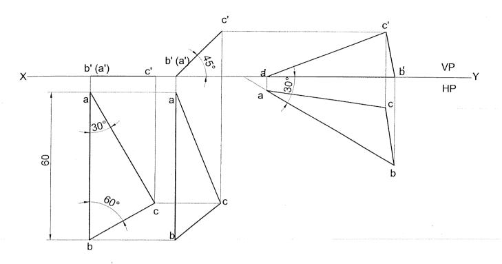
**Problem 7** An isosceles triangular plate of negligible thickness has base 25mm long and altitude 35mm. It is so placed on HP such that in the front view it is seen as an equilateral triangle of 25mm sides with the side that is parallel to VP is inclined at 45° to HP. Draw its top and front views. Also determine the inclination of the plate with the reference plane.
