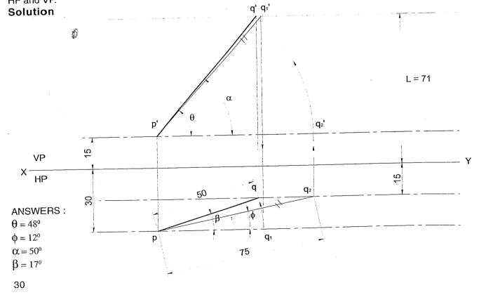
**Problem 9** A line AB 60 mm long has one of its extremities 20 mm informt of VP and 15 mm above HP. The line is inclined at 25° to HP and 40° to VP. Draw its top and front views. **Solution**
