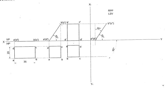
**Problem 14** A rectangular lamina of 35mm x 20mm rests on HP on one of its shorter edges. The lamina is rotated about the edge on which it rests till it appears as a square in the top view. The edge on which the lamina rests is inclined 30° to VP. Draw its projections and find its inclination to HP.
