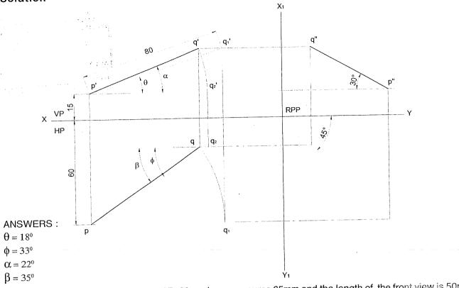
**Problem 48** The top view of a line AB, 80mm long measures 65mm and the length of the front view is 50mm. The end A is on HP and 15mm infront of VP. Draw the projections
