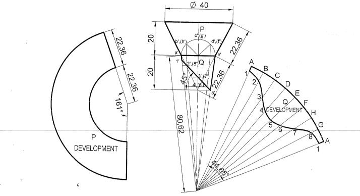
**P.roblem 50** A funnel is made of sheet metal. The funnel tapers from 60 mm. to 30 mm. diameters to a height of 25 mm. and then forms to a cylinder with a height of 50 mm. Bottom of funnel is beveled off completely at an angle of 45° to axis Draw the development of funnel.
