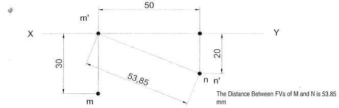
**Problem 14** A point P is on HP and 30 mm in front of VP. Another point Q is on VP and 40 mm above HP. The distance between their projectors parallel to XY line is 50 mm. Find the distance between their front and top views of the points P and Q.
