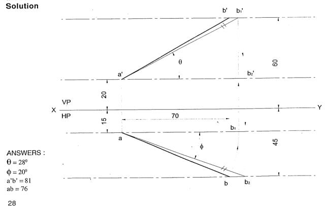
**Problem 5** The top view PQ of a straight line is 70 mm and makes an angle of 60° with XY line. The end Q is 10 mm infront of VP and 30 mm above the HP. The difference between the distances of P and Q above the HP is 45 mm. draw the projections. Determine its true length and true inclinations with HP and VP.
