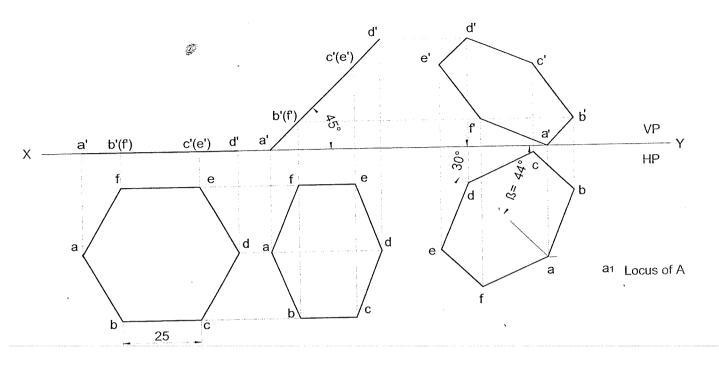
**Problem 42** A hexagonal lamina of sides 25mm rests on one of its corners on HP. The lamina makes 45° to HP and he diagonal passing through the corner on which it rests appears to be inclined at 30° to VP. Draw its projections. **Solution**
