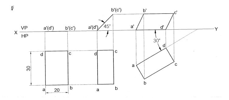
**Problem 13** A rectangular lamina of 35mm x 20mm rests on HP on one of its shorter edges. The lamina is rotated about the edge on which it rests till it appears as a square in the top view. The edge on which the lamina rests being parallel to both HP and VP. Draw its projections and find its inclinations to HP and VP.
