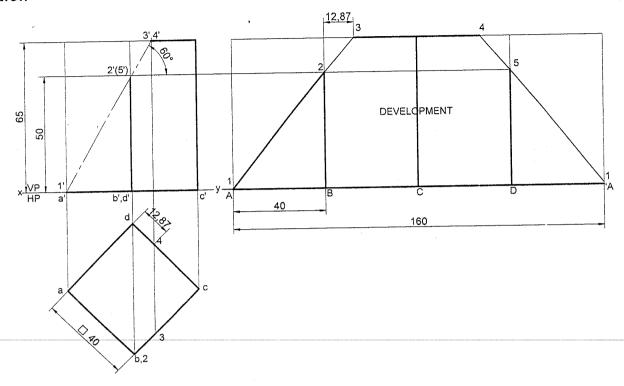
**Problem 4** A square prism of 30mm side of the base and height 50mm is resting with its base on HP such that one of its vertical faces is inclined at 40° to VP. It is cut as shown in the following front view figure. Draw the development of the lateral surface of the prism.
