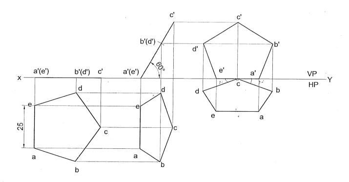
**Problem 29** A pentagonal lamina of edges 25mm is resting on VP with one of its sides such that the surface makes an angle of 60° with VP. The edge on which it rests is inclined at 45° to HP. Draw its projections.
