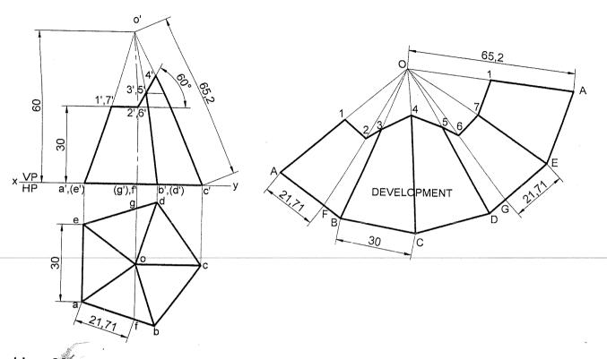
**Problem 26** A pentagonal pyramid of 30mm edges of base and 50mm height rests vertically with one of its base edges parallel to VP and nearer to it. It is cut as shown in following figure. Draw the development of the lateral surfaces of the upper portion of the pyramid. **Solution**
