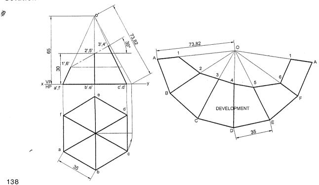
**Problem 29** A hexagonal pyramid 25 mm side of base and axis 65 mm long is resting on its base on HP with one of the edges of the base parallel to VP. It is cut by a vertical section plane at a distance of 8 mm from the axis towards right solution.
