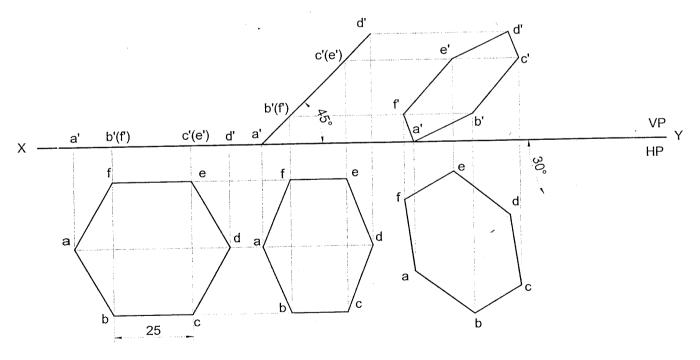
**Problem 43** A hexagonal lamina of sides 25mm rests on one of its sides on VP. The lamina makes 45° to VP and the side on which it rests makes 45° to HP. Draw its projections. **Solution**
