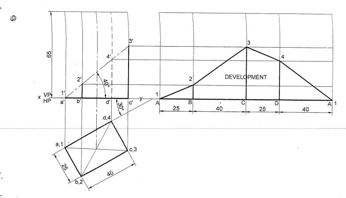
**Problem 10** Draw the development of the truncated portion of the lateral faces of a pentagonal prism of 20mm sides of base and 50mm height standing vertically with one of its rectangular faces parallel to VP and nearer to it so as to produce a one piece development. The inclined face of the truncated prism is 30° to its axis and passes through the right extreme corner of the top face of the prism.
