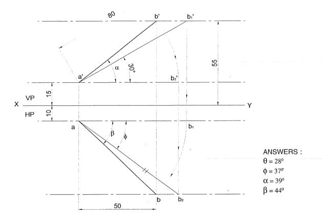
**Problem 46** The end A of a line AB is in HP and 25mm in front of VP. The end B is 10 mm in front of VP and 50mm above HP. The distance between the end projectors when measured parallel to the line of intersection of HP & VP is 80 mm. Draw the projections of the line AB and determine its true length and true inclinations with HP & VP. **Solution**
