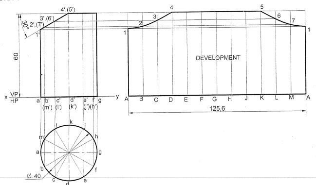
**Problem 36** A cone of base diameter 60mm and height 70mm is resting on its base on HP. It is cut as shown in the following figure. Draw the development of the lateral surface of the remaining portion of the cone.
