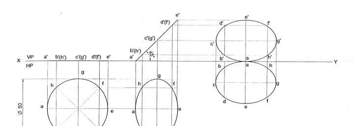
**Problem 48** A circular lamina of 50mm diameter rests on HP such that one of its diameters is inclined at 30° to VP and 45° to HP. Draw its top and front views in this position. **Solution**
