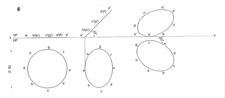
**Problem 47** A circular lamina of 50mm diameter is standing with one of its points on the rim on HP and the lamina inclined at 45° to HP. The diameter at right angles to the diameter which is passing through the point on which the lamina rests is parallel to VP. Draw its projections. **Solution**
