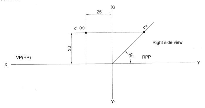
**Problem 45** A point is lying on VP, 10 mm below HP & 30 mm behind / in front / from LPP. Draw its projections and name the side view.
