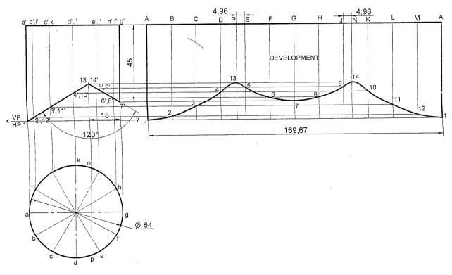
**Problem 33** A vertical cylinder of base diameter 50mm and axis length 60mm is cut by a two planes which are perpendicular to VP and inclined at 45° to HP and passing through either side the centre point of the top face. Draw the development of the lateral surface of the cylinder. **Solution**
