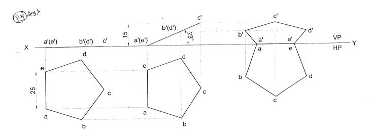
**Problem 26** A regular pentagonal lamina of 25mm side is resting on one of its corners on HP while the side opposite to this corner touches VP. If the lamina makes an angle of 60° with HP and 30° with VP, draw the projections of the lamina.
