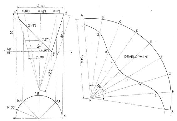
**Problem 43** A hexagonal pyramid of 30mm sides of base with a side of base parallel to VP. Draw the development of the lateral surfaces of the retained portion of the pyramid which is shown by dark lines in the following figure. **Solution**
