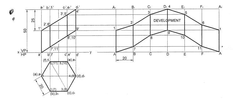
**Problem 16** A hexagonal prism of base side 25mm and height 55mm is resting on HP on its base, such that one of its base edges is parallel to VP. The prism is cut in this position as shown in the following front view. Draw the development of the lateral surface of the prism.
