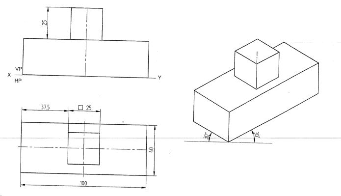
**Problem 42** Two rectangular plates are placed centrally with dimensions (lxbxh)100mmx60mmx20mm and 100mmx40mmx20mm such that longer edges are parallel. Draw the isometric projection of the combination **Solution**
