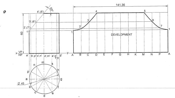
**Problem 32** Following figure shows the front view of a model of a steel chimney of diameter 60mm made from a flat thin sheet metal fitted over an inclined plane roof. Develop the portion of the chimney.
