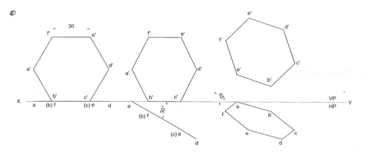
**Problem 40** A hexagonal lamina of sides 25mm rests on one of its sides on HP. The lamina makes 45° to HP and the side on which it rests makes 30° to VP. Draw its projections. **Solution**
