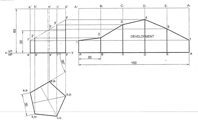
**Problem 12** A pentagonal prism of 30mm side of base and height 50mm lies with its base on HP such that one of the rectangular faces is inclined at 40° to VP. It is cut to the shape of a truncated pyramid with the truncated surface inclined at 30° to the axis so as to pass through a point on it 30mm above the base. Develop the truncated portion of the prism so as to produce a one piece development.
