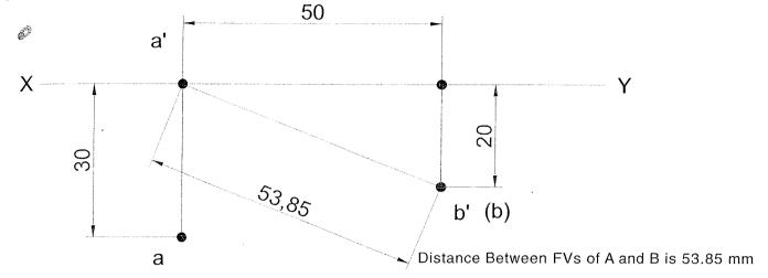
**Problem 38** A point P is on HP and 30 mm in front of VP. Another point Q is on VP and 40 mm above HP. The distance between their projectors parallel to XY line is 50mm. Find the distance between their front and top views of the points P and Q.
