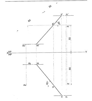
**Problem 25** A straight line PQ inclined at  $40^{\circ}$  to VP has pq = 60 mm and p'q' = 50 mm. The end P is both in HP and VP, and 40 mm to the right of left profile plane
