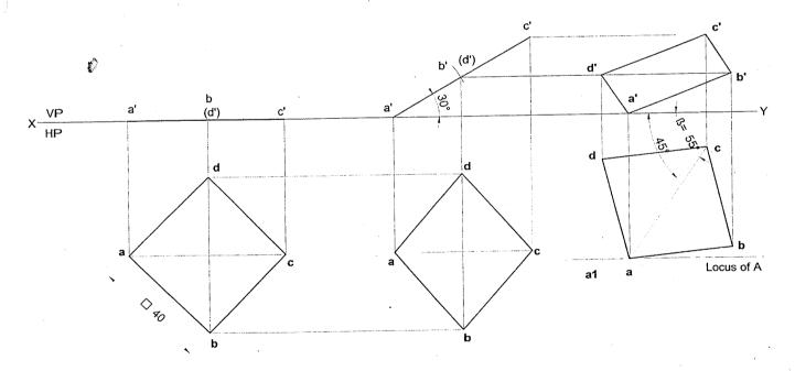
HP and the **blem 10** A square lamia ABCD of 40mm side rests on corner C such that the diagonal AC appears to be at 45°to The two sides BC and CD containing the corner C make equal inclinations with HP. The surface of the lamina makes with HP. Draw its top and front views.
