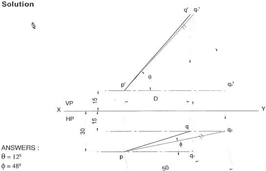
**Problem 28** A straight line AB measuring 80 mm long has the end A in the HP and 25 mm in front of the VP. Its mid point M is 25 mm above the HP and 40 mm in front of the VP. Draw the projections of the line and determine the inclination of the line with HP and VP.
