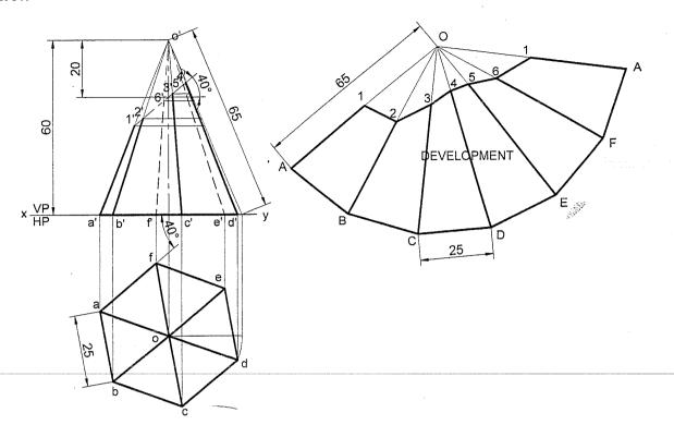
**Problem 28** A hexagonal pyramid of sides 35mm and altitude 65mm is resting on HP on its base with two of the base sides perpendicular to VP. The pyramid is cut by a plane inclined at 30° to HP and perpendicular to VP and is intersecting the axis at 30mm above the base. Draw the development of the remaining portion of the pyramid.
