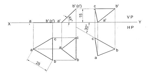
**Problem 6** A 30°-60° setsquare of 60mm longest side is so kept such that the longest side is in HP, making an angle of 30° with VP. The set square itself is inclined at 45° to HP. Draw the projections of the setsquare. **Solution**
