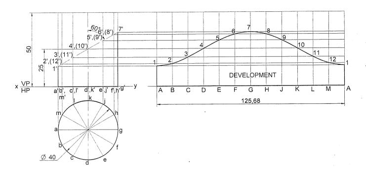
**Problem 40** Develop the lateral surface of the cylinder of 40mm diameter and height 60mm cut in the following way. **Solution**
