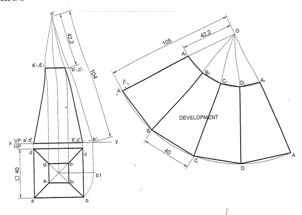
**Problem 21** A square pyramid of 25mm base edge and 50mm height rests with its base on HP with all of its base edges equally inclined to VP. It is cut by a plane perpendicular to VP and inclined to HP at 60°, passing through the extreme right corner of base. Draw the development of the lateral surface of the pyramid. **Solution**
