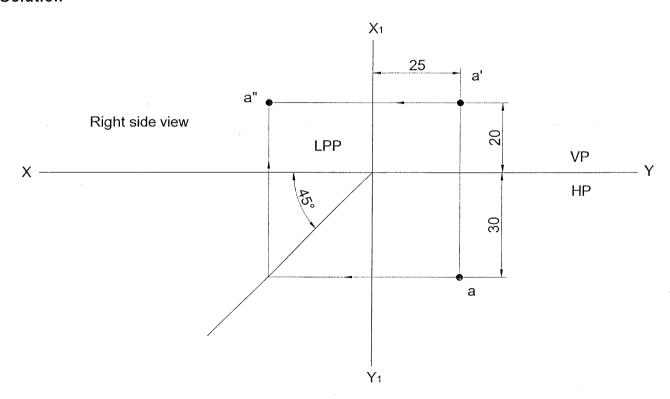
**Problem 43** A point is 40 mm behind VP, 20 mm above HP and 30 mm in front / behind / from LPP.Draw its projections and name the side view.
