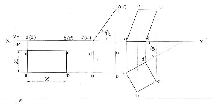
**Problem 15** A rectangular lamina of sides 20mm x 25mm has an edge in HP and adjoining edge in VP, is tilted such that the front view appears as a rectangle of 20mm x 15mm. The edge, which is in VP, is 30mm from the right profile plane. (a) Draw the top view, front view and the left profile view in this position. (b) Find its inclinations with the corresponding principal planes.
