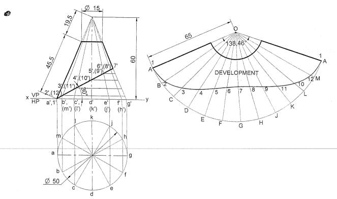
**Problem 46** A cone of base diameter 50mm and height 60mm is resting with its base on HP. It is cut, as shown in the following front view of which is as shown in figure. Draw the development of the lateral surface of it. **Solution**
