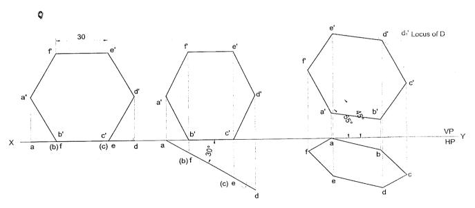
**Problem 39** A hexagonal lamina of sides 30mm is resting on HP with one of its corners in VP and its surface inclined at an angle of 30° with VP. The diagonal passing through that corner which is in VP appears to be inclined at 4**g**° to HP. Draw the projections of the lamina.
