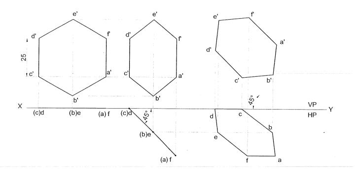
**Problem 44** A hexagonal lamina of sides 25mm rests on one of its sides on VP. The side opposite to the side on which it rests is 30mm infront of VP & the side on which it rests makes 45° to HP. Draw its projections. Also determine the inclination of the lamina with the reference plane.
