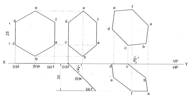
**Problem 45** A hexagonal lamina of sides 25mm rests on one of its corners on HP. The corner opposite to the corner on which it rests is 35mm above HP and the diagonal passing through the corner on which it rests is inclined at 30° to VP. Draw its projections. Find the inclination of the surface with HP.
