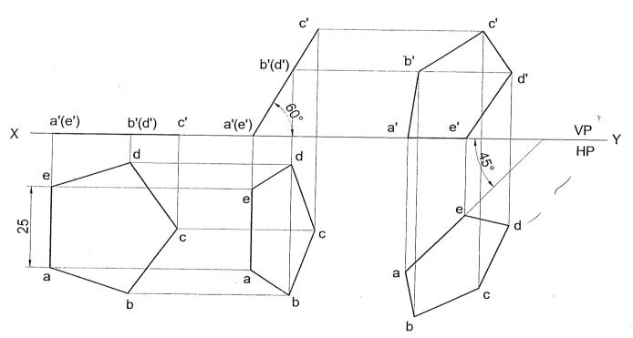
**Problem 20** A pentagonal lamina of edges 25mm is resting on HP with one of its corners such that the plane surface makes an angle of 60° with HP. The two of the edges containing the corner on which the lamia rests make equal inclinations with HP. When the edge opposite to this corner make an angle of 45° with VP and nearer to the observer, draw the top and front views of the plane lamina in this position.
