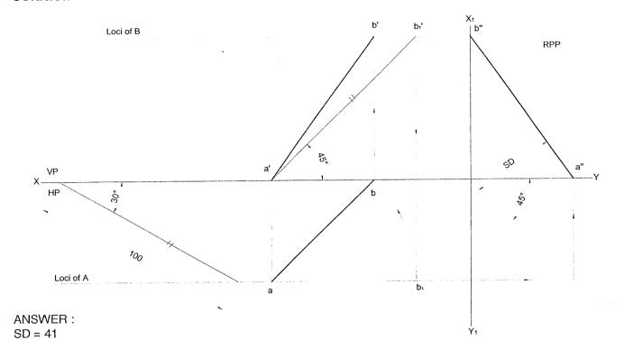
**Problem 16** A line AB 100 mm long is inclined to HP at 45° and inclined to VP at 30°. Draw front and top views of line and determine their lengths. Also determine the perpendicular distance of end Q from both HP and VP. **Solution**
