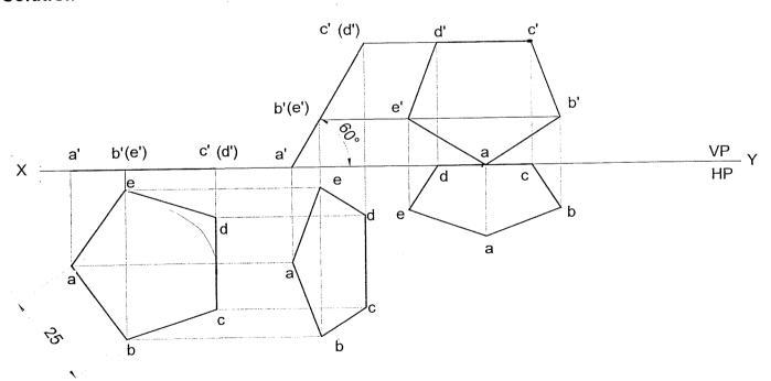
**Problem 27** A pentagonal lamina having edges 25mm is placed on one of its corners on HP such that the surface makes an angle 30° with HP and perpendicular bisector of the edge passing through the corner on which the lamina rests appears to be inclined at 30° to VP. Draw the top and front views of the lamina. **Solution**
