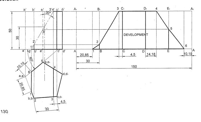
**Problem 13** A pentagonal prism of base sides 30mm and axis length 60mm rests with its base on HP and an edge of the base inclined at 45° to VP. It is cut by a plane perpendicular to VP, inclined at 40° to HP and passing through a point on the axis, at a distance of 30 mm from the base. Develop the remaining surfaces of the truncated prism.
