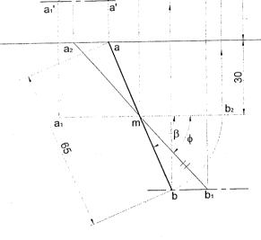
**Problem 36** A straight line PQ is inclined at 45° to HP and 30° to VP. The point P is in HP and the point Q is in VP. The length of the straight line is 65 mm. draw the projections of the straight line AB.
