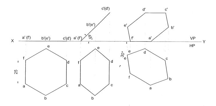
**roblem 41** A hexagonal lamina of sides 25mm rests on one of its corners on HP. The lamina makes 45° to HP and e diagonal passing through the corner on which it rests is inclined at 30° to VP. Draw its projections. **olution**
