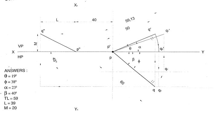
**Problem 26** A line has one end 30 mm in front of VP and 15 mm above HP and the other end is 15 mm in front of VP and is above HP. Length of the line is 60 mm. Top view of the line is 40 mm long. Draw the two views of the line and obtain the inclination of the line with HP and VP.
