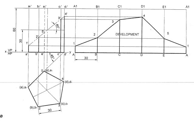
**Problem 14** A pentagonal prism of base sides 20mm and height 40mm is resting with its base on HP and base edge parallel to the VP. The prism is cut as shown in the following front view. Draw the development of the lateral surface of the prism.
