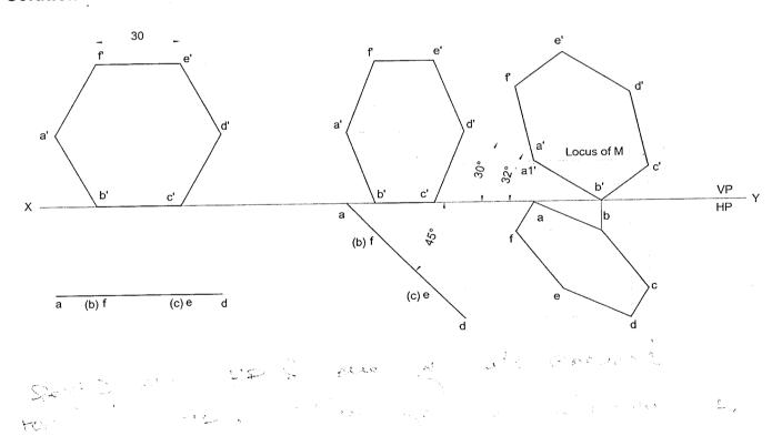
**Problem 33** Draw the top and front views of a hexagonal lamina of 30mm sides having two of its edges parallel to both vertical and horizontal planes and one of its edges is 10mm from each of the planes of projection. The surface of the lamina is inclined at an angle of 60° to the HP.
