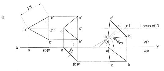
**Problem 4** A triangular plane figure of sides 25mm is resting on HP with one of its corners, such that the surface of the lamina makes an angle of 60° with HP. If the side opposite to the corner on which the lamina rests makes an angle of 30° with VP, draw the top and front views in this position.
