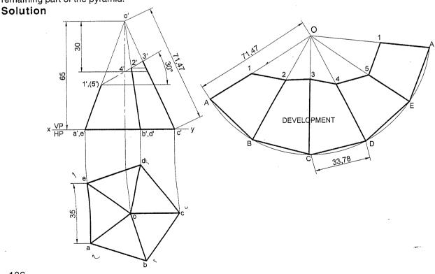
**Problem 25** A pentagonal pyramid, 30mm sides, with a side of base perpendicular to VP. Draw the development of the lateral surfaces of the retained portion of the pyramid shown by the dark lines in the following figure. **Solution**
