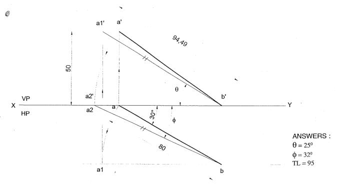
**Problem 15** Draw the projections of a straight line AB, 100 mm long, inclined at 45° to HP and 30° to VP. The end A is in HP and the end B is in VP. Find the shortest distance between the straight line AB and the line of intersection of planes of projection.
