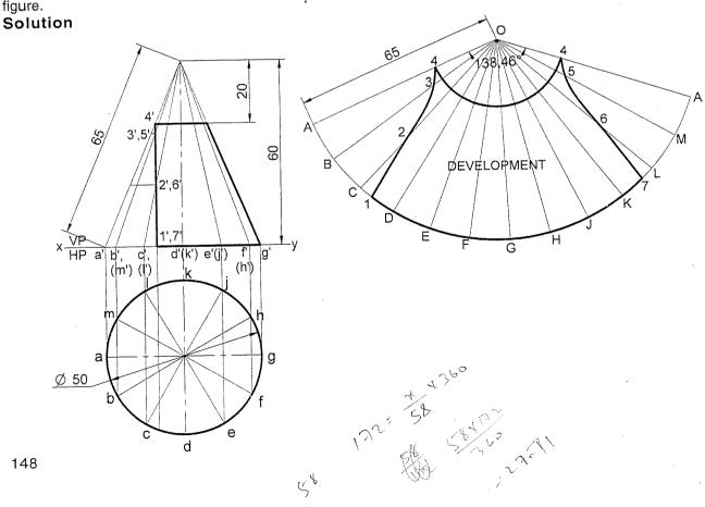
**Problem 49** A funnel is to be made of sheet metal. The funnel tapers from 40 mm to 20 mm diameter to a height of 20 mm and from 20 mm to 15 mm diameter, for the next 20 mm height. The bottom of the funnel is beveled off to a plane inclined at 45° to the axis. Draw the development of the funnel. **Solution**
