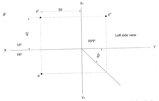
**Problem 16** The point P is 45 mm above HP, 60 mm behind VP and 30 mm from RPP. Draw the three principles view of the point. Also state the quadrant in which it lies.
