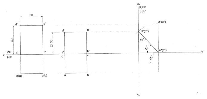
**Problem 18** A rectangular plate of negligible thickness of size 35x20mm has one of its shorter edges in VP with that edge inclined at 40° to HP. Draw the top view if its front view is a square of side 20mm. **Solution**
