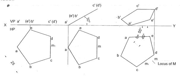
**Problem 24** A pentagonal lamina of sides 25mm is having a side both on HP and VP. The corner opposite to the side on which it rests is 15mm above HP. Draw the top and front views of the lamina. **Solution**
