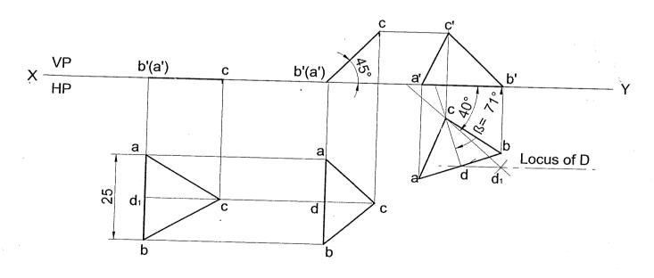
**Problem 3** A triangular lamina of 25mm sides rests on one of its corners on VP such that the median passing through the corner on which it rests is inclined at 30° to HP and 45° to VP. Draw its projections.
