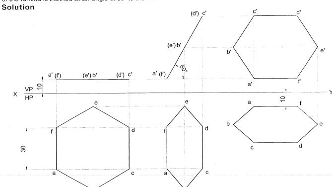
**Problem 34** A regular hexagonal lamina of sides 30mm is lying in such a way that one of its sides touches both the reference planes. If the lamina makes 60° with HP, draw the projections of the lamina.
