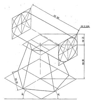
**Problem 5** Following figure shows the front view of combination of solids consisting a cut sphere and frustums of a cone and a square pyramid. Draw the Isometric projection of the combination of solids. **Solution**
