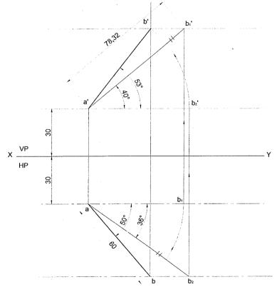
**Problem 35** The top view of the line AB 80 mm long, measures 65 mm. The mid point of the line is 60 mm in front of VP and 70 mm above HP. The point A is in the VP. Draw its projections and find its inclinations.
