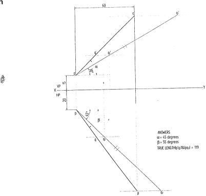
**Problem 32** The top view ab of a straight line AB is 60 mm long and makes an angle of 30<sup>0</sup> with the XY line. The end A is in VP and 30 mm above HP. The end B is 65 mm above HP. Draw the projections of the line AB and determine i) length of the front view ii) its true length and true inclinations with the reference planes.
