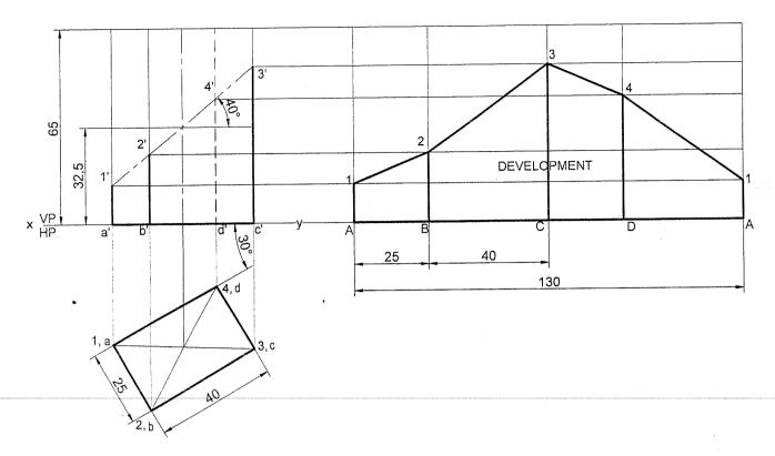
**Problem &** A rectangular prism of base 30mm x 20mm and height 60mm rests on HP on its base with the longer base side inclined at 40° to VP. It is cut by a plane inclined at 45° to HP, perpendicular to VP and bisects the axis. Draw the development of the lateral surface of the prism.
