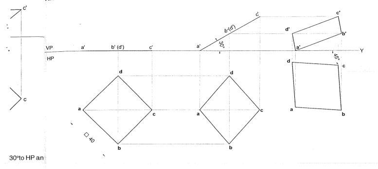
**pblem 11** The top view of a square lamia of side 30mm is a rectangle of sides 30mm x 20mm with the longer side he rectangle being parallel to both HP and VP. Draw the top and front views of the square lamina. What is the lination of the surface of the lamina with HP and VP?
