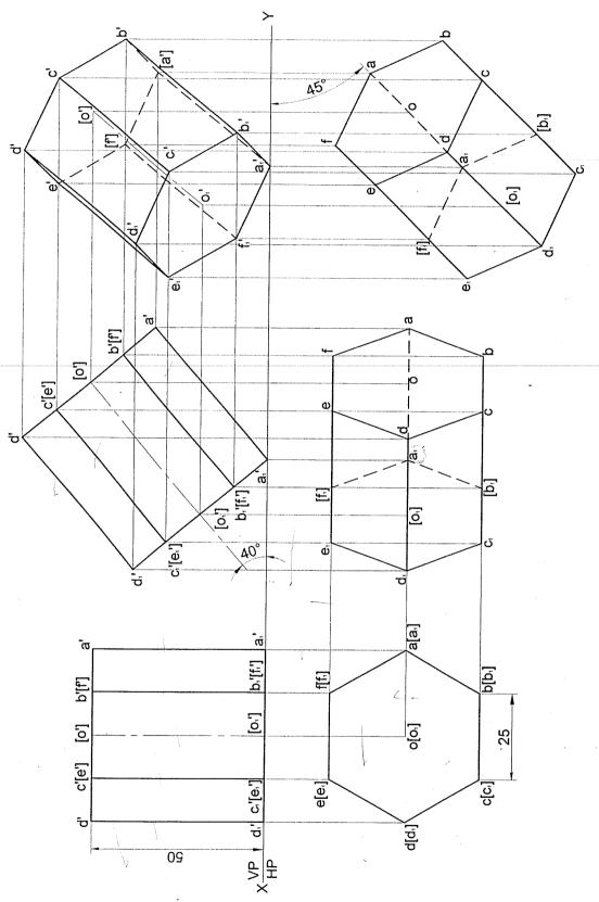
roblem 12 A hexagonal prism 25 mm sides of base and 50 mm axis length rests on HP on one of its corners of the ise such that the two base edges containing the corner on which it rests make equal inclinations with HP. Draw the ojections of the prism when the axis of the prism is inclined to HP at 40° and to VP at 30°. olution
