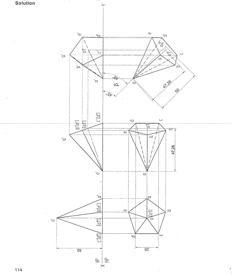
**Problem 39** A hexagonal pyramid 25 mm sides of base and 50 mm axis length rests on HP on one of its slant edges. Draw the projections of the pyramid when the axis appears to be inclined to VP at 45°. **Solution**
