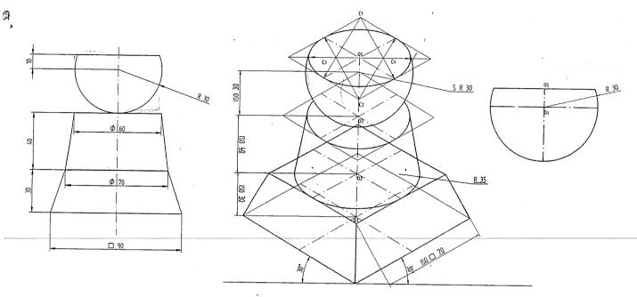
**Problem 6** The frustum of a square pyramid of sides 40mm and height 60mm rest on the centre of the top of a square block of side 60mm and height 20mm. The base edges of the pyramid are parallel to the top edges of the square block. Draw the isometric projection of the combination of the solids. **Solution**
