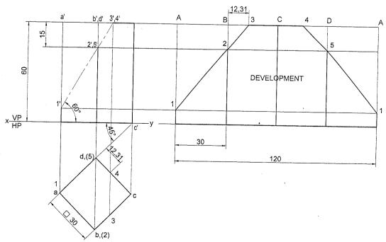
**Problem 3** A square prism of base side 40mm and axis length 65mm is resting on HP on its base with all the vertical faces being equally inclined to VP. It is cut by an inclined plane 60° to HP and perpendicular to VP and is passing through a point on the axis at a distance 15mm from the top face. Draw the development of the lower portion of the prism.
