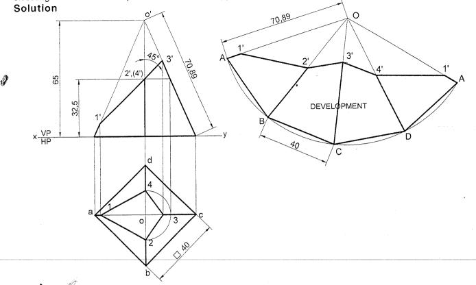
**Problem 10** A frustum of a square pyramid has its base 40 mm sides, top 16 mm sides and height 60mm, its axis is vertical and a side of its base is parallel to VP. Draw the projections of the frustum and show the development of the lateral surfaces of it.
