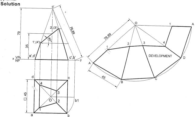
**Problem 1.9** A square pyramid base 40mm side and axis 65mm long has its base on HP and all the edges of the base are equally inclined to VP. It is cut to with an inclined section plane so as the truncated surface at 45° to its axis, bisecting it. Draw the development of the truncated pyramid.
