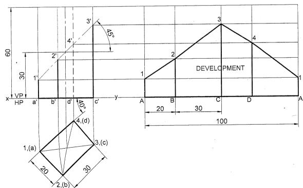
**Problem 9** A rectangular prism of base size 25mm×40mm and axis length 65mm is resting on HP on its base with the longer side of base inclined at 30° to VP. It is cut by a plane inclined at 40° to HP and perpendicular to VP and passes through the extreme left corner of base. Draw the development of the lateral surface of the remaining portion of the prism.
