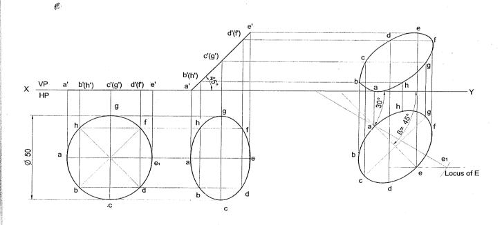
**Problem 49** A circular lamina inclined to the VP appears in the front view as an ellipse of major axis 30mm and minor axis 15mm. The major axis is parallel to both HP and VP. One end of the minor axis is in both the HP and VP. Draw the projections of the lamina and determine the inclination of the lamina with the VP. **Solution**
