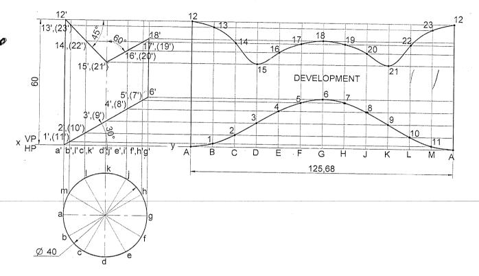
**Problem 38** A cone of base diameter 60mm and height 70mm is resting on its base on HP. It is cut as shown in the following figure. Draw the development of the lateral surface of the remaining portion of the cone. **Solution**
