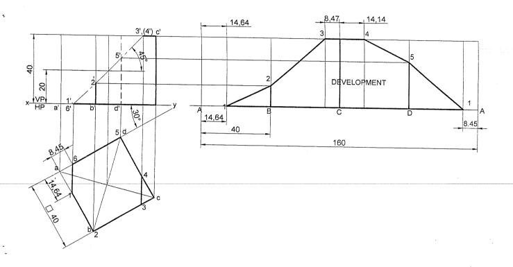
**Problem &** A square prism of base side 35mm rests with its base on HP and two faces equally inclined to VP. Draw the development of the lateral surfaces of the retained portions of the cut prism shown by dark lines in the Fig. **Solution**
