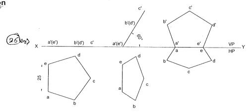
**Problem 25** A pentagonal lamina of sides 25mm is having a side both on HP and VP. The surface of the lamina is inclined at an angle of 60° with HP. Draw the top and front views of the lamina.
