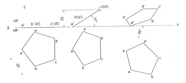
**Problem 22** A pentagonal lamina of sides 25mm is resting on one of its edges on HP with the corner opposite to that edge touching VP. This edge is parallel to VP and the corner, which touches VP, is at a height of 15mm above HP. Draw the projections of the lamina and determine the inclinations of the lamina with HP and VP and the distance at which the parallel edge lies from VP.
