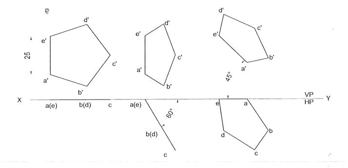
**Problem 30** A pentagonal lamina having edges 25mm is placed on one of its corners on VP such that the surface makes an angle 30° with VP and perpendicular bisector of the edge passing through the corner on which the lamina rests appears to be inclined at 30° to HP. Draw the top and front views of the lamina.
