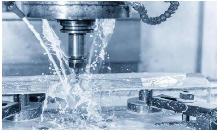
Figure 1. Application of cutting fluids on drilling
