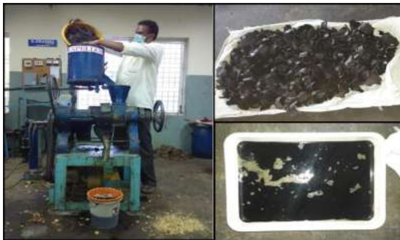
Mechanical Expeller and expelled cakes of Garcinia seed
