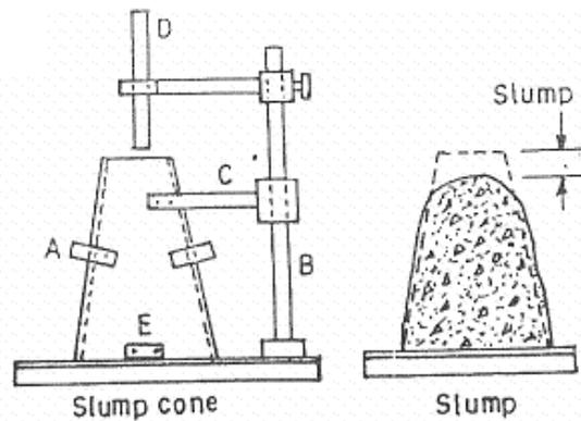
The slump cone and slump.
