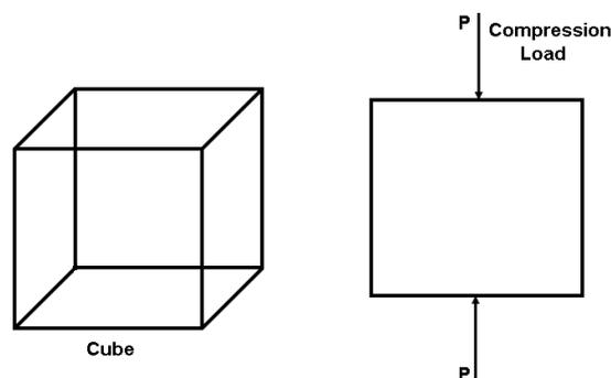
**Calculations:** Compressive strength of cement = load / area = .....  $\text{N/mm}^2$
