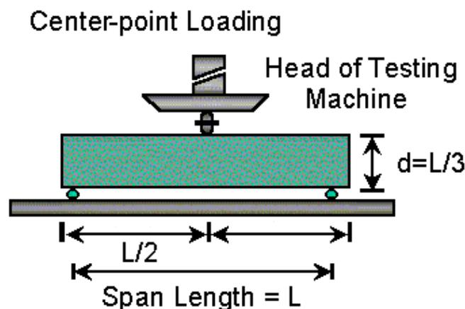
**Flexural Testing on concrete**
